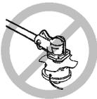
**⚠ WARNING:** The blade continues to spin after the throttle is released or engine is turned off. The coasting blade can throw objects or seriously cut you if accidentally touched. Stop the blade by contacting the right hand side of the coasting blade with material already cut.
