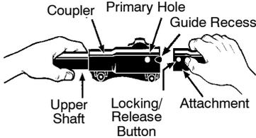
**WARNING:** Make sure the locking/release button is locked in the primary hole and the knob is securely tightened before operating the unit. All attachments are designed to be used in the primary hole unless otherwise stated in the applicable attachment instruction manual. Using the wrong hole could lead to serious injury or damage to the unit.
