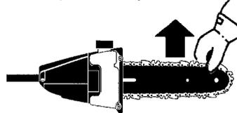
7. Use the screwdriver end of the bar tool to move chain around guide bar.
