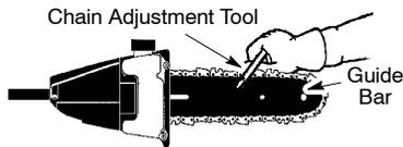
2. Loosen bar clamp nut until it is finger tight against the bar clamp.
