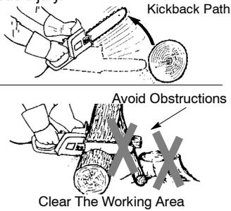
**⚠ WARNING:** Avoid kickback which can result in serious injury. **Kickback** is the backward, upward or sudden forward motion of the guide bar occurring when the saw chain near the upper tip of the guide bar contacts any object such as a log or branch, or when the wood closes in and pinches the saw chain in the cut. Contacting a foreign object in the wood can also result in loss of chain saw control.
