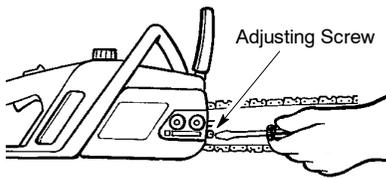
5. Check the tension by lifting the chain from the guide bar. Remove some of the stiffness in the chain by pulling down and letting go of the chain several times.
