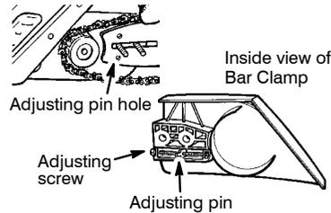
8. Secure the guide bar and bar clamp with the bar clamp nuts; tighten finger tight *only*.
