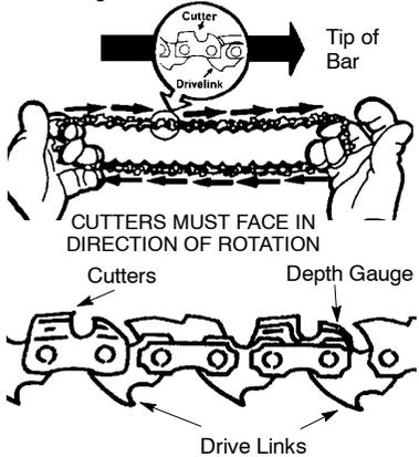
6. Place chain around the sprocket and fit the drive links into the guide bar groove and then into the teeth of the sprocket in the tip of the guide bar.
