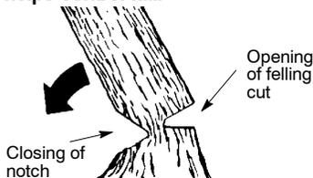
**NOTE:** Before felling cut is complete, use wedges to open the cut when necessary to control the direction of fall. To avoid kickback and chain damage, use wood or plastic wedges, but never steel or iron wedges.
