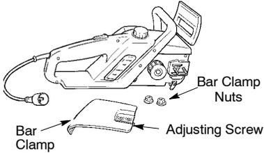
4. Turn the adjusting screw counter-clockwise to move the adjusting pin almost as far as it will go to the rear. Do not remove the adjusting screw from the bar clamp.
