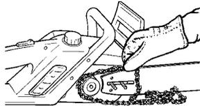
7. Hold the guide bar against the saw frame and install the bar clamp. Be sure adjusting pin is in the adjusting pin hole in the bar.
