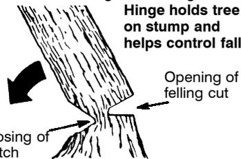
**NOTE:** Before felling cut is complete, use wedges to open the cut when necessary to control the direction of fall. Use wood or plastic wedges, but never steel or iron, to avoid kickback and chain damage.
