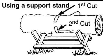
**REMOVING A PINCHED SAW
