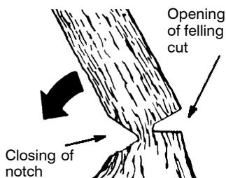
**NOTE:** Before felling cut is complete, use wedges to open the cut when necessary to control the direction of fall. Use wood or plastic wedges, but never steel or iron, to avoid kickback and chain damage.
