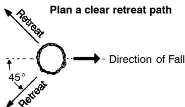
**WARNING:** Do not cut near buildings or electrical wires if you do not know the direction of tree fall, at night since you will not be able to see well, or during bad weather such as rain, snow, or strong winds. etc.
