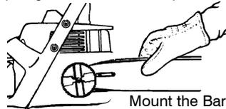
5. Prepare the chain by checking the proper direction. Without following the illustration it is easy to place the chain on the saw in the wrong direction. Use the illustration of the chain to determine the proper direction.
