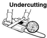
**Undercutting** involves cutting on the underside of the log with top of saw against the log. When undercutting use light upward pressure. Hold saw firmly and maintain control. The saw will tend to push back toward you.
