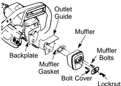
1. Loosen and remove the locknut from the bolt cover.
