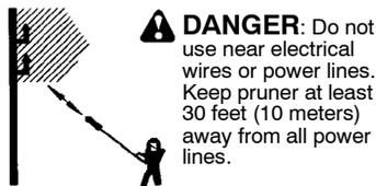
**DANGER:** Do not use near electrical wires or power lines. Keep pruner at least 30 feet (10 meters) away from all power lines.
