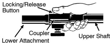
3. While securely holding the motor housing and upper shaft, pull the attachment straight out of the coupler.
