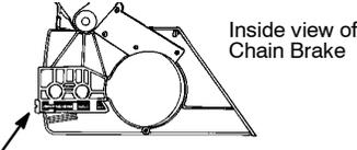
4. Turn the adjusting screw by hand counter-clockwise until the adjusting pin just touches the stop. This should allow the pin to be near the correct position. Further adjustment may be necessary as you mount the bar.
