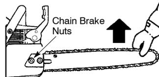
**WARNING:** If the saw is operated with a loose chain, the chain could jump off the guide bar and result in serious injury.
