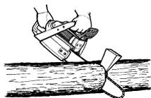
Turn saw **OFF** and use a plastic or wooden wedge to force cut open.
