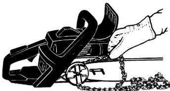
Place chain onto the sprocket
