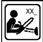
Measured maximum kickback value, with and without chain brake, for the bar and chain combination on the label.
