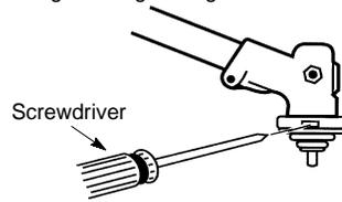
9. Tighten blade nut firmly with a wrench while holding screwdriver in position.
