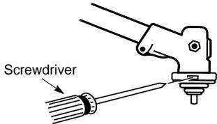
7. While holding the screwdriver in position, thread trimmer head onto the shaft in the direction shown on the decal (counterclockwise). Tighten until secure.
