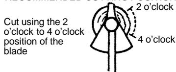
**WARNING:** The operator or others must not try to clear away cut material with the engine running or the blade turning to avoid serious injury. Stop engine and blade before removing materials wrapped around blade or shaft.
