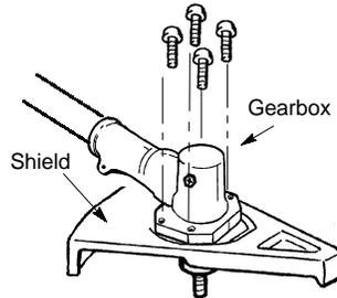
2. Insert and thread the 4 mounting screws through the holes of the gearbox and the metal shield. Tighten evenly and securely with the hex wrench provided.
