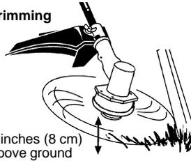
**SCALPING** - The scalping technique removes unwanted vegetation down to the ground. Hold the bottom of the trimmer head about 3 in. (8 cm) above the ground and at an angle. Allow the tip of the line to strike the ground around trees, posts, monuments, etc. This technique increases line wear.
