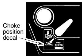
8. Pull starter rope sharply until engine runs, but no more than 6 pulls. If the engine doesn't start after 6 pulls (at the HALF CHOKE position), move the choke lever to the FULL CHOKE position and press the primer bulb 6 times. Squeeze and hold the throttle trigger and pull the starter rope 2 more times. Move the choke lever to the HALF CHOKE position and pull the starter rope until the engine runs, but no more than 6 pulls. If the engine doesn't start, repeat procedure 2 additional times.
