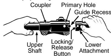
**WARNING:** Make sure the locking/release button is locked in the primary hole and the knob is securely tightened before operating the unit. All attachments are designed to be used in the primary hole.
