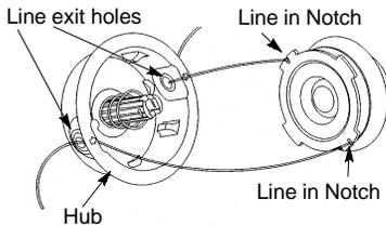
5. Wind the line evenly and tightly onto the spool. Wind in the direction of the arrows found on the spool.
