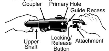
**WARNING:** Make sure the locking/release button is locked in the primary hole and the knob is securely tightened before operating the unit.
