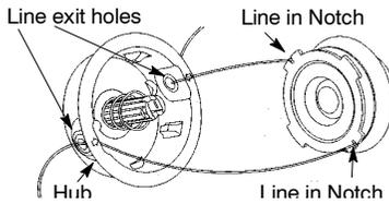
5. Wind the line evenly and tightly onto the spool. Wind in the direction of the arrows found on the spool.
