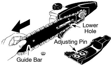
13. Install bar clamp nut and finger tighten only. Do not tighten any further at this point. Proceed to the CHAIN ADJUSTMENT section.
