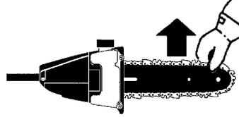
7. Use the screwdriver end of the bar tool to move chain around guide bar.
