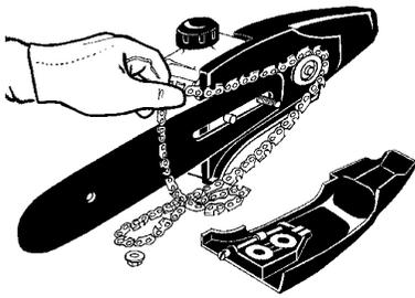
8. Place chain over sprocket, fitting the drive links in the sprocket.
