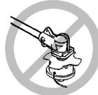
**⚠ WARNING:** The blade continues to spin after the throttle is released or engine is turned off. The coasting blade can throw objects or seriously cut you if accidentally touched. Stop the blade by contacting the right hand side of the coasting blade with material already cut.
