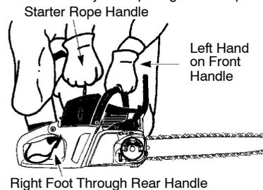
**WARNING:** Do not attempt to throw or drop-start the chain saw. Doing so will put the operator at risk of serious injury due to loss of control of the chain saw.
