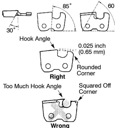
**WARNING:** Maintain the proper hook angle according to the manufacturer's specifications for the chain you are using. Improper hook angle will increase the chance of kickback which can result in serious injury.
