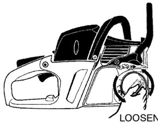
3. Remove clutch cover and plastic shipping spacer (if present).
