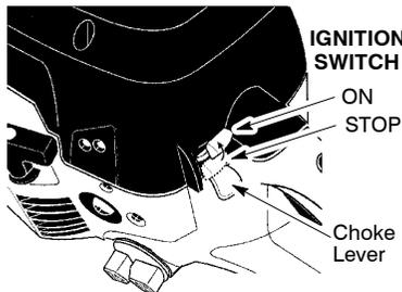
1. Move ON/STOP switch to the ON position.
