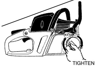
5. Push lever on bar knob down to return lever to closed/locked position.
