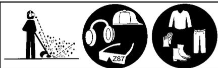
Blade/trimmer line can throw objects violently. You can be blinded or injured. Always wear hearing protection and safety glasses marked Z87. Always wear head protection, heavy, long pants, long sleeves, boots and gloves.
