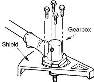
2. Insert and thread the 4 mounting screws through the holes of the gearbox and the metal shield. Tighten evenly and securely with the hex wrench provided.
