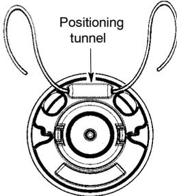
5. Insert ends of line one at a time through the line exit tunnels.
