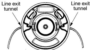
7. Correctly installed line will be the same length on both ends.
