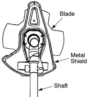
1. Place the metal shield under the gearbox, and align the screw holes.
