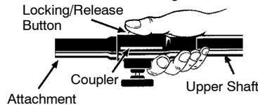
3. While securely holding the engine and upper shaft, pull the attachment straight out of the coupler.
