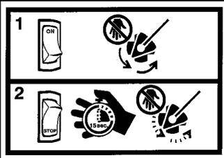
**⚠ WARNING:** The blade continues to spin after the trigger is released or engine is turned off. The coasting blade can throw objects or seriously cut if accidentally touched. Stop the blade by contacting the right hand side of the coasting blade with material already cut.
