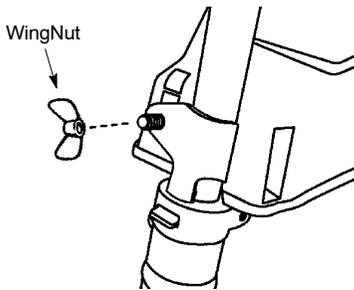
**NOTE:** If your unit has a plastic cover over the threads on the threaded shaft, remove the covering to expose the threads. Before installing the trimmer head, make sure the dust cup and retaining washer are positioned on the gearbox as shown below.
