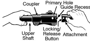
**WARNING:** Make sure the locking/release button is locked in the primary hole and the knob is securely tightened before operating the unit. All attachments are designed to be used in the primary hole unless otherwise stated in the applicable attachment instruction manual. Using the wrong hole could lead to serious injury or damage to the unit.
