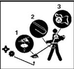
**⚠ WARNING:** Always use a metal shield and dust cup in the order shown when using blades. Always use a handlebar and shoulder strap. Ensure handlebar remains installed at all times.
