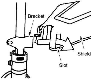
4. Reinstall wing nut and tighten securely.
