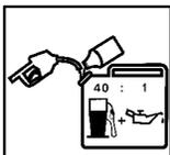
Use unleaded gasoline and two-stroke oil mixed at a ratio of 40:1 (2.5%).
