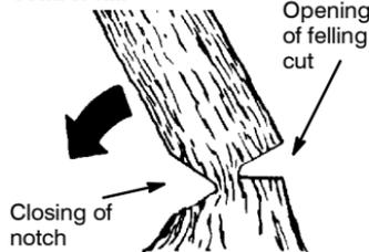
**NOTE:** Before felling cut is complete, use wedges to open the cut if necessary to control the direction of fall. To avoid kickback and chain damage, use wood or plastic wedges, but never steel or iron wedges.
