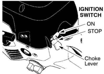
1. Move ON/STOP switch to the ON position.
