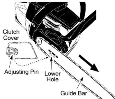
12. Install bar nuts and finger tighten only. Once the chain is tensioned, you will need to tighten bar nuts.
