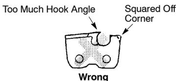
**WARNING:** Maintain the proper hook angle according to the manufacturer's specifications for the chain you are using. Improper hook angle will increase the chance of kickback which can result in serious injury.
