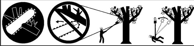
**⚠ WARNING:** Avoid kickback which can result in serious injury. Kickback is the backward, upward or sudden forward motion of the guide bar occurring when the chain near the upper tip of the guide bar contacts any object such as a log or branch, or when the wood closes in and pinches the chain in the cut. Contacting a foreign object in the wood can also result in loss of control.
