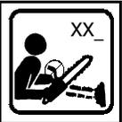
Measured maximum kickback value, without chain brake, for the bar and chain combination on the label.
