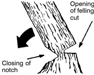
**NOTE:** Before felling cut is complete, use wedges to open the cut when necessary to control the direction of fall. To avoid kickback and chain damage, use wood or plastic wedges, but never steel or iron wedges.
