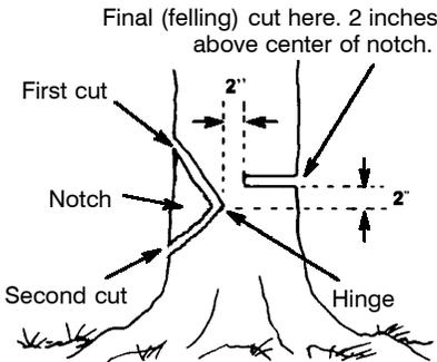
**Hinge holds tree on stump and helps control fall**
