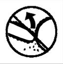
**WARNING!** Contacting the guide bar tip with any object should be avoided; tip contact may cause the guide bar to move suddenly upward and backward, which may cause serious injury.
