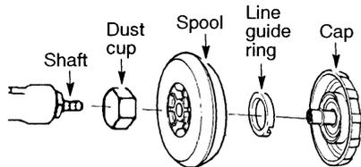
Use a pre-wound spool or refill spool with line. If using a pre-wound spool, remove tape strip from line and spool.
