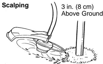
**MOWING** - Your trimmer is ideal for mowing in places conventional lawn mowers cannot reach. In the mowing position, keep the line parallel to the ground. Avoid pressing the head into the ground as this can scalp the ground and damage the tool.
