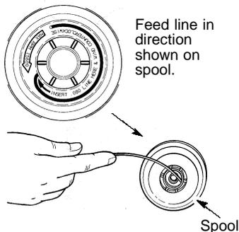
2. Insert one end of line into center cavity of empty spool. Ensure line will feed into spool in the direction shown on the spool (counterclockwise).
