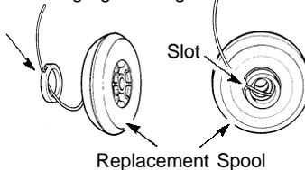
3. Rest guide ring on spool and place line through slot. Allow line to extend 4 - 6 inches (10 - 15 cm) from center of spool.
