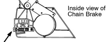
4. Turn the adjusting screw by hand counterclockwise until the adjusting pin just touches the stop. This should allow the pin to be near the correct position.
