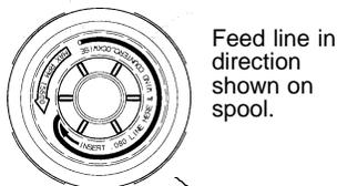
2. Insert one end of line into center cavity of empty spool. Ensure line will feed into spool in the direction shown on the spool (counterclockwise).
