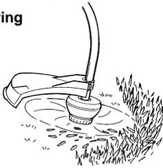
**SWEEPING** - The fanning action of the rotating line can be used for a quick and easy clean up. Keep the line parallel to and above the surfaces being swept and move the tool from side to side.
