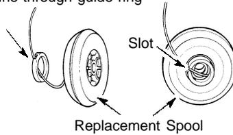
3. Rest guide ring on spool and place line in slot. Allow line to extend 4 - 6 inches (10 - 15 cm) from center of spool.
