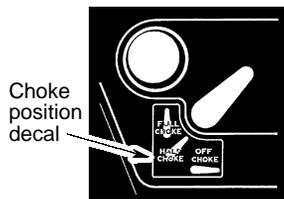
7. Pull starter rope sharply until engine runs, but no more than 6 pulls. If the engine doesn't start after 6 pulls (at the HALF CHOKE position), move the choke lever to the FULL CHOKE position and press the primer bulb 6 times. Squeeze and hold the throttle trigger and pull the starter rope 2 more times. Move the choke lever to the HALF CHOKE position and pull the starter rope until the engine runs, but no more than 6 pulls. If the engine doesn't start, repeat procedure 2 additional times.
