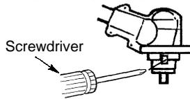
7. While holding the screwdriver in position, thread trimmer head onto the shaft in the direction shown on the decal (counter-clockwise). Tighten until secure.
