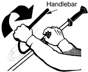
2. Rotate handlebar/clamp counterclockwise toward engine until clamp falls into groove of base.
