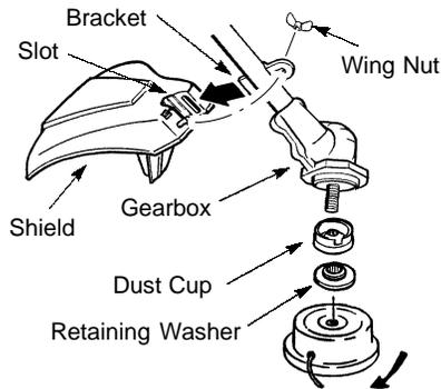
**NOTE:** Make sure all parts are properly installed as shown in the illustration before installing the trimmer head.
