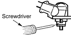
9. Tighten blade nut firmly with a wrench while holding screwdriver in position.
