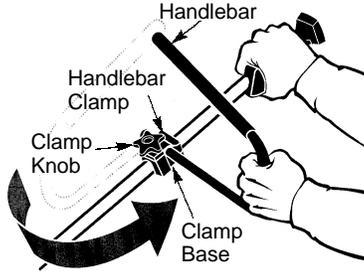
3. Place the handlebar in a comfortable position.
