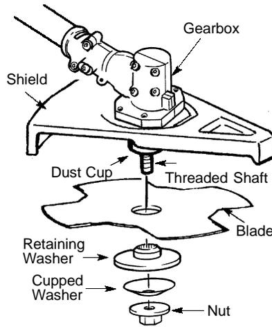
**NOTE:** Make sure all parts are in place as illustrated, and the blade is sandwiched between the dust cup and the retaining washer. There should be no space between the blade and the dust cup or the retaining washer.
