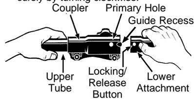
**WARNING:** Make sure the locking/release button is locked in the primary hole and the knob is securely tightened before operating the unit. All attachments are designed to be used in the primary hole.
