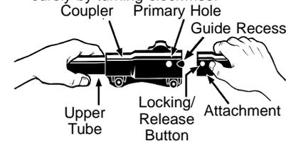
**WARNING:** Make sure the locking/release button is locked in the primary hole and the knob is securely tightened before operating the unit.
