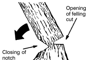
**NOTE:** Before felling cut is complete, use wedges to open the cut when necessary to control the direction of fall. To avoid kickback and chain damage, use wood or plastic wedges, but never steel or iron wedges.
