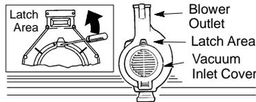
3. Gently tilt the handle of the screwdriver toward the back of the unit to release the latch while pulling up on the vacuum inlet cover with your other hand.
