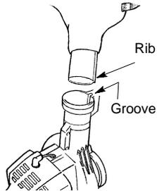
5. Insert the elbow tube into the blower outlet. Make sure elbow tube rib is aligned with the blower outlet groove.
