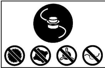
**⚠ DANGER:** Use only specified trimmer head, spool, and 0.080 inch (2 mm) recommended trimmer line. Never use blades, flailing devices, wire, rope, string, etc. Unit is designed for line trimmer use only. Failure to follow these instructions may result in serious injury.
