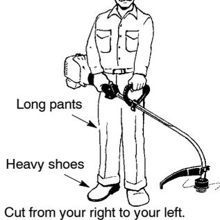
**WARNING:** Always wear eye protection. Never lean over the trimmer head. Rocks or debris can ricochet or be thrown into eyes and face and cause blindness or other serious injury.
