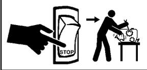
Always stop unit and disconnect spark plug before cleaning or servicing.
