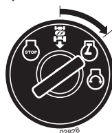
ENGINE "ON" POSITION (NORMAL OPERATING)
