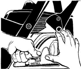
TENSIONING LEVER IN INSTALL POSITION
