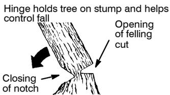
**NOTE:** Before felling cut is complete, use wedges to open the cut when necessary to control the direction of fall. To avoid kickback or chain damage, use wood or plastic wedges, but never steel or iron wedges.
