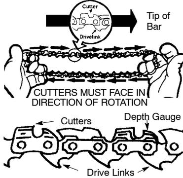
8. Place chain over and behind clutch, fitting the drive links in the clutch drum sprocket.
