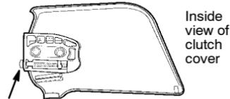
Adjustment located on clutch cover
