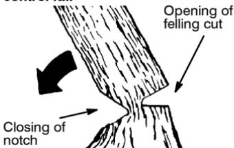
**NOTE:** Before felling cut is complete, use wedges to open the cut if necessary to control the direction of fall. To avoid kickback and chain damage, use wood or plastic wedges, but never steel or iron wedges.
