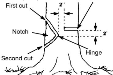
• After removing the wood from the notch, make the felling cut on the opposite side of the notch. This is done by making a cut about two inches (5 cm) higher than the center of the notch. This will leave enough uncut wood between the felling cut and the notch to form a hinge. This hinge will help prevent the tree from falling in the wrong direction.
