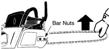
6. Use the screwdriver end of the bar tool to move chain around guide bar.
