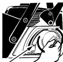
Tensioning Lever LOOSEN
