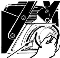
5. While lifting tip of guide bar, turn adjustment knob handle clockwise to clamp bar. Tighten until bar is clamped securely. **Hand tighten securely; do not use tools to tighten!**
