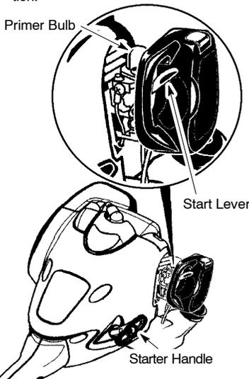
4. Pull starter rope handle sharply until engine starts and runs.
