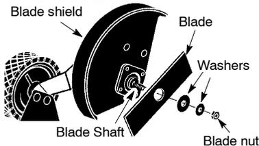
5. Install new blade onto blade shaft.
