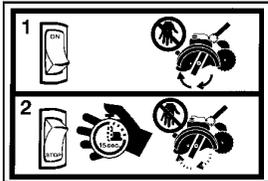
**⚠ DANGER:** Blade moves momentarily after the trigger switch is released.
