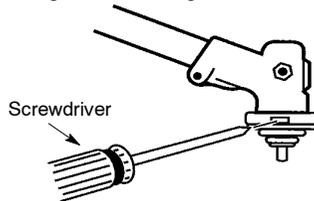
3. While holding the screwdriver in position, remove blade nut by turning clockwise.
