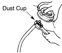
2. Remove trimmer head by turning counterclockwise (looking from bottom of unit).
