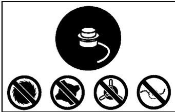
**⚠ DANGER:** Use only specified trimmer head, spool, and 0.080 inch (2 mm) recommended trimmer line. Never use blades, flailing devices, wire, rope, string, etc. This attachment is designed for line trimmer use only. Failure to follow these instructions may result in serious injury.
