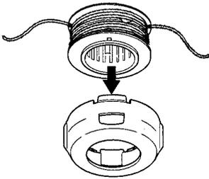
10. Insert the ends of the lines through exit holes in the sides of the cover.
