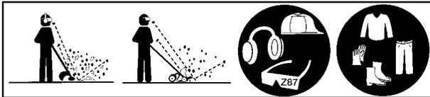
Blade/trimmer line can throw objects violently. You can be blinded or injured. Always wear hearing protection and safety glasses marked Z87. Always wear head protection, heavy, long pants, long sleeves, boots and gloves.
