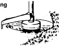
**SWEEPING** - The fanning action of the rotating line can be used for a quick and easy clean up. Keep the line parallel to and above the surfaces being swept and move the tool from side to side.
