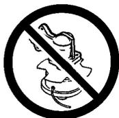
**⚠ WARNING:** The blade continues to spin after the trigger is released or engine is turned off. The coasting blade can throw objects or seriously cut you if accidentally touched. Stop the blade by contacting the right hand side of the coasting blade with material already cut.
