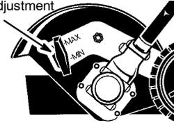
1. Loosen the depth adjustment knob.
