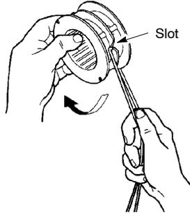
7. With your finger between the lines, wrap the lines evenly and firmly around the spool in a clockwise direction.
