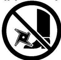
**⚠ WARNING:** Inspect the area to be cultivated before starting the unit. Remove all debris and hard and sharp objects such as rocks, vines, branches, rope, string, etc.
