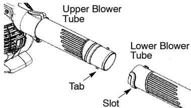
4. Slide the lower blower tube onto the upper blower tube.
