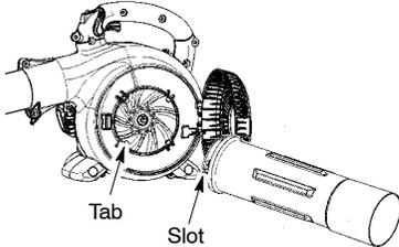
5. Push the upper vacuum tube into the vacuum inlet. Turn the tube counterclockwise until a click is felt to secure the tube to the blower unit.
