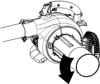
6. Align slanted end of lower vacuum tube as shown. Firmly push lower vacuum tube into upper vacuum tube.
