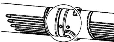
6. To remove the tubes, turn the knob counterclockwise to loosen the tubes; remove the tubes.
