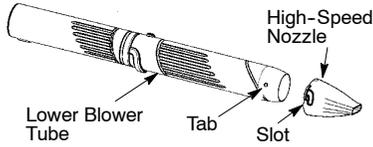
2. Slide the nozzle onto the lower blower tube.
