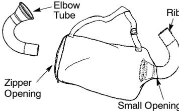
**NOTE:** Make sure edge of the small opening is flush against the flared area of the elbow tube, and the rib on the elbow tube is on the bottom.
