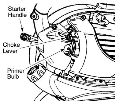
5. Pull starter rope handle sharply until engine sounds as if it is trying to start, but do not pull rope more than 6 times.
